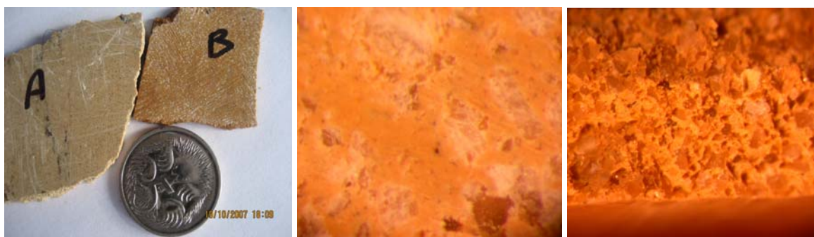
Figure 2: Two asbestos vinyl tiles and their magnified edges.
