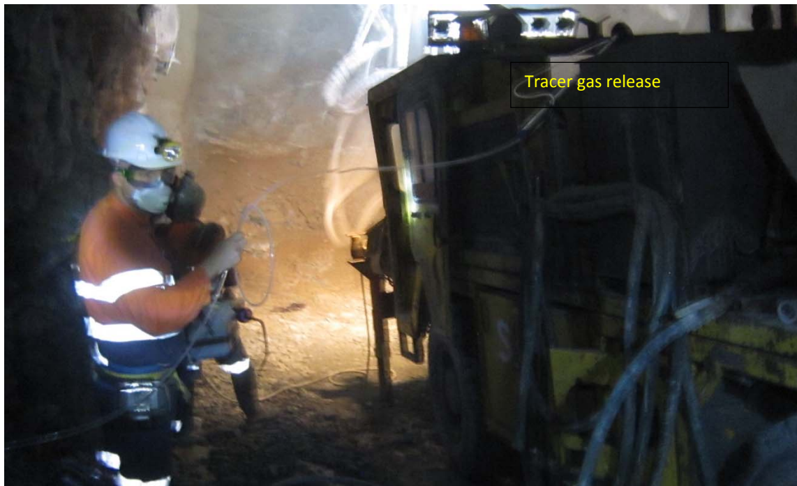
FIG 1 – Tracer gas released into Spraymech exhaust
