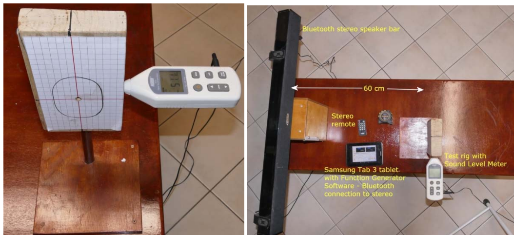
Figure 22 Sound Level Meter inserted in muff /plug test block (L), Test rig ( R )
