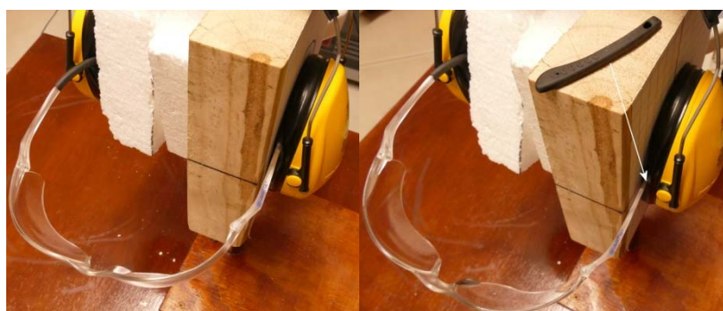
Figure 26 Yellow muff and safety glasses with and without the comfort rubber on the frame
