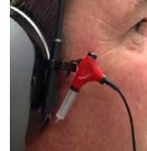
Figure 3: Dual-element microphone attached to the earmuff test probe
