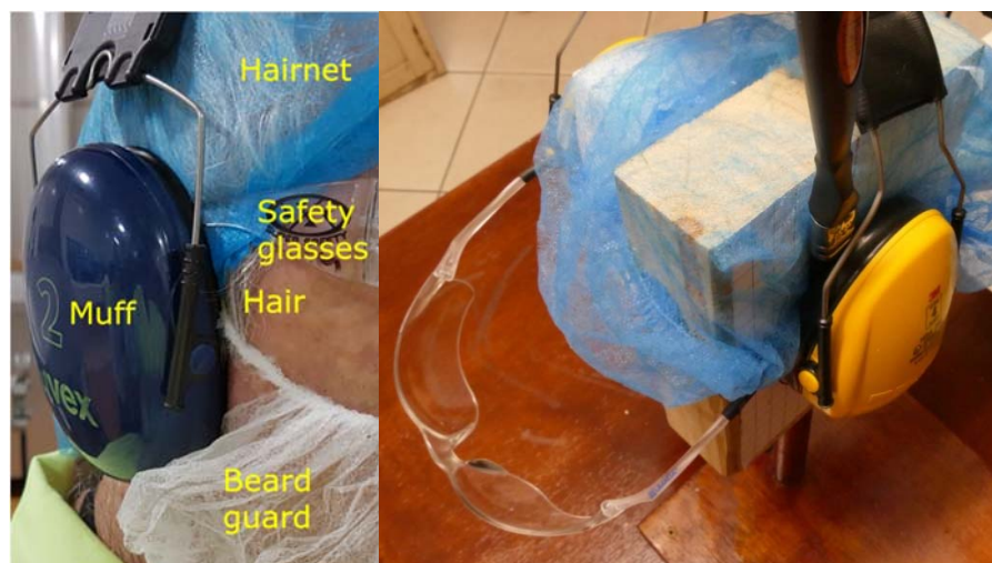
Figure 19 Ear muff and hairnet with beard guard, safety glasses and hair; laboratory test rig
