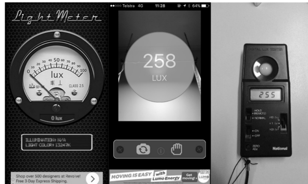
Figure 2. Mobile phone apps and illuminance meter. Left to right (a) light meter application for Android, (b) light meter application for iOS and (c) National lux tester
